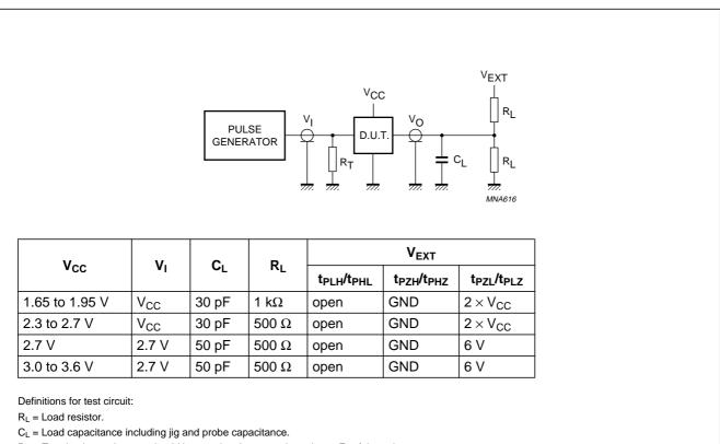
$R_T$  = Termination resistance should be equal to the output impedance  $Z_0$  of the pulse generator.
